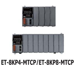
4-slot Intelligent Ethernet I/O Expansion Unit (Modbus TCP Protocol)
